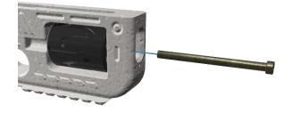
Grease the center hole of the cylinder, and use a 65mm M5 bolt to secure the cylinder assembly in the frame. The ball bearing should provide enough resistance to firmly and securely click into each barrel position, but still smoothly rotate between barrels without having to force. You may need to add a washer between the cylinder and the front of the frame depending on tolerances and whether or not material was removed from sanding.
